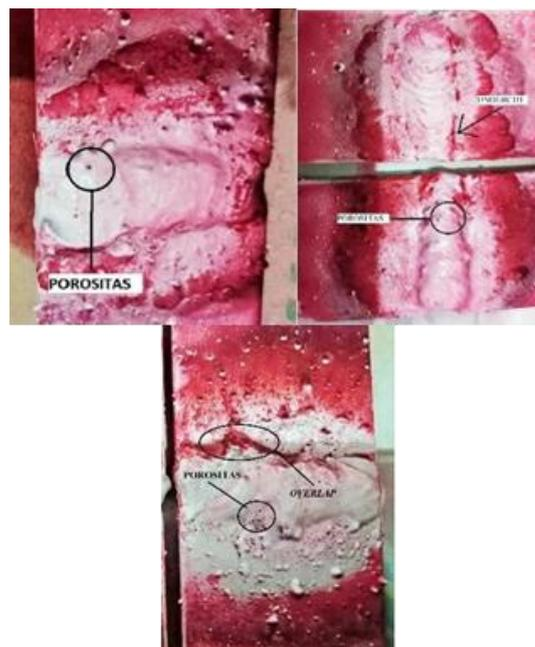
Gambar 2. Penetrant test
