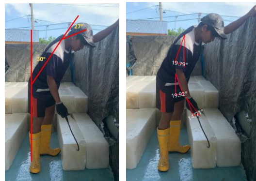
Fig. 2. Analysis of work posture in the process of moving ice blocks using the REBA method: (a) initial posture when pulling ice blocks; (b) continued posture when moving ice blocks to the transport area..
