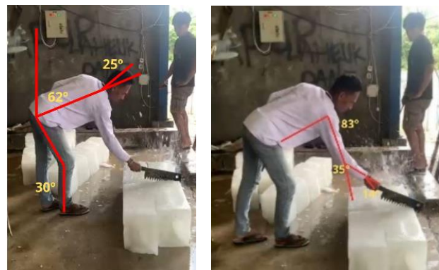
Fig. 4. Analysis of the third worker's working posture during the ice block cutting process using the REBA method: (a) initial posture when cutting the ice block; (b) continued posture during the cutting process.
