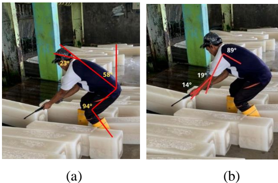
Fig. 1. Analysis of worker 1's work posture in the process of moving ice blocks using the REBA method. (a) posture when pulling ice blocks from the mold; (b) posture when positioning ice blocks for transfer.
